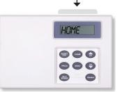
Inserted into the top of the Control Panel is a Quick Reference card that provides information on the basic operation of the FloLogic System.
